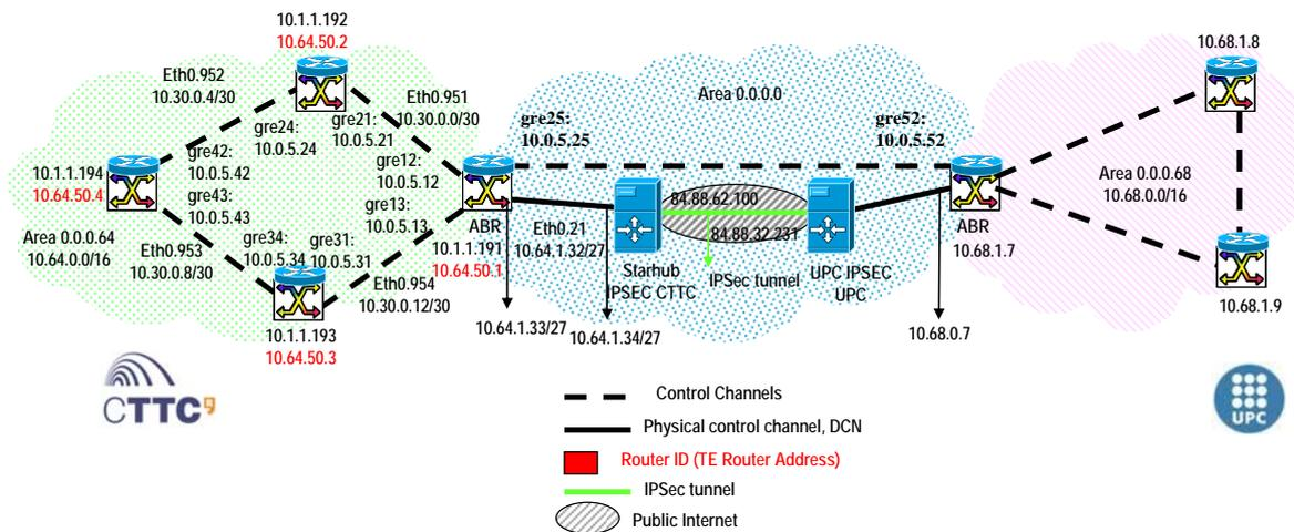
Figure JA8-1 IP connectivity and DCN design between UPC CARISMA and CTTC ADRENALINE testbeds
