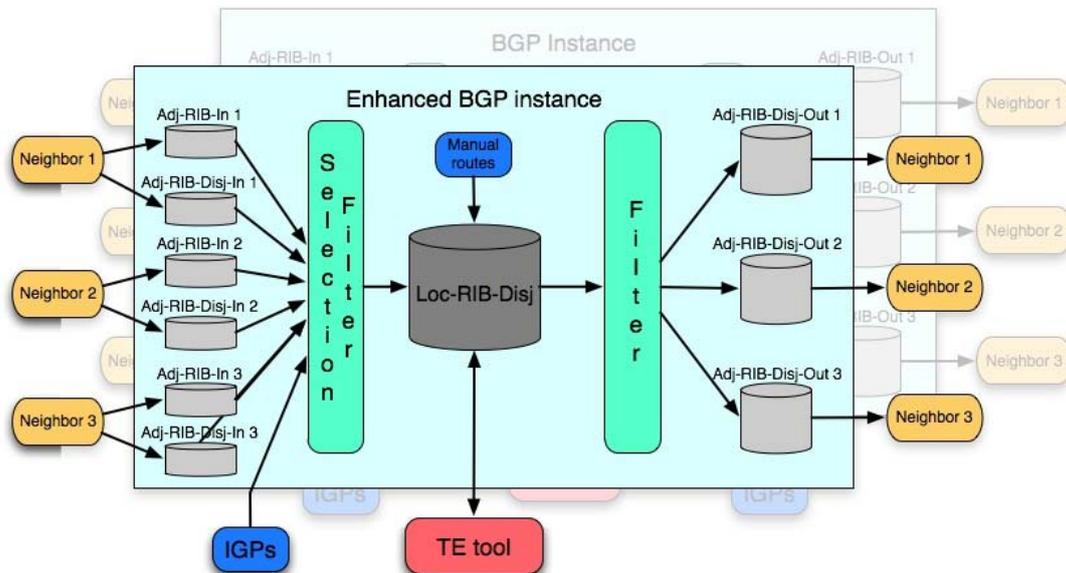
Figure JA2-4 Proposed selection mechanism scheme for disjoint AS\_PATH dissemination
