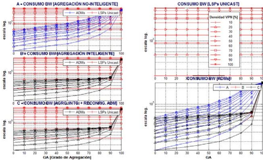
Fig JA5-1. Bandwidth consumption in Tiscali network for 25% of VPLS member density
