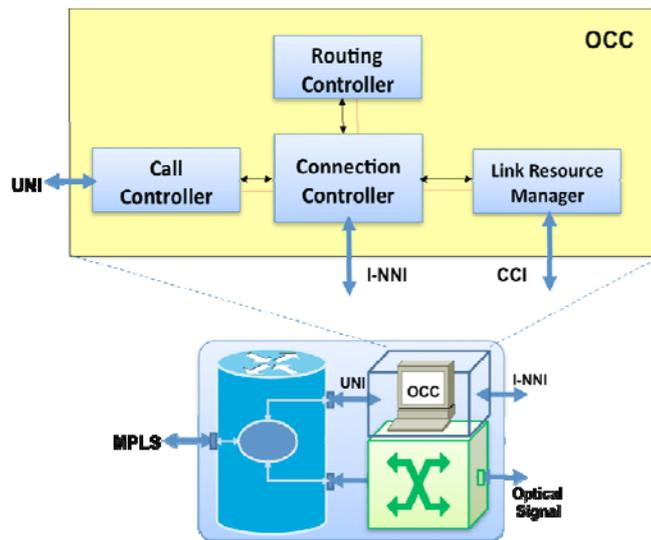
Figure JA4-2 Modules of the border nodes
