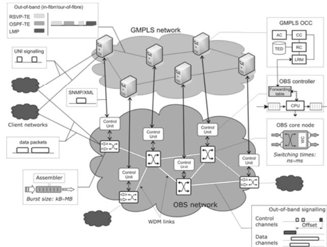
*Figure JA9-1 The OBS Network Architecture with an Interoperable GMPLS/OBS Control Plane. Legend: LRM: Link Resource Manager, AC: Admission Controller, RC: Routing Controller, CC: Connection Controller, TED: Traffic Engineering Database.*
