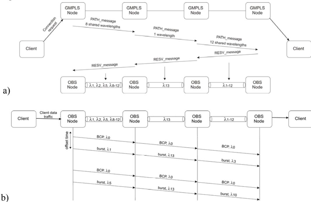
Figure JA9-2 Example of the GMPLS-controlled overlay logical network consisting of a) TE tunnels between sources and destinations, and b) wavelength selection at each OBS node.
