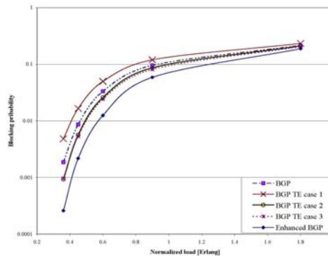
Figure JA2-1 Blocking probability vs. Normalized Load
