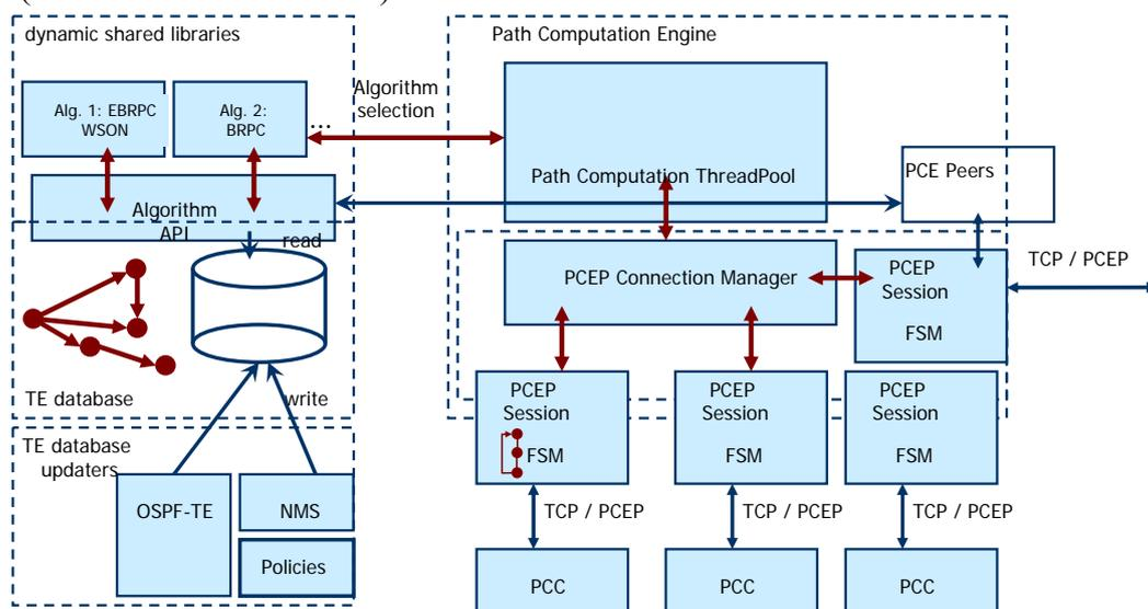
Figure JA1-1 PCE functional architecture
