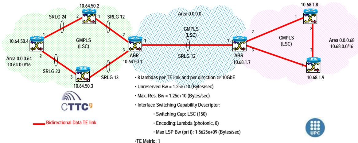
Figure JA8-2 Emulated TE link connectivity between UPC CARISMA and CTTC ADRENALINE testbeds
