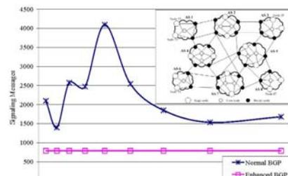
The efficiency of the modified BGP protocol was also evaluated in terms of needed overhead for re-convergence of the protocol in order to accommodate any changes in the TE state of the disseminated paths. Fig. JA2-2 illustrates the result. The stable operation of the **Enhanced BGP** is evident, whereas the normal BGP operation has unpredictable overhead. Next, Fig.
