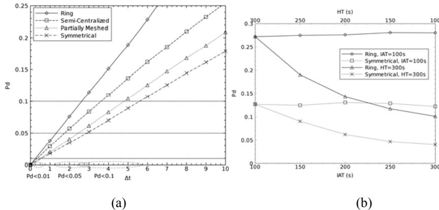
Fig. JA7-3 (a) Comparison of  $P_d$  for each topology under study, (b)  $P_d$  with constant IAT and HT for ring and symmetrical topologies
