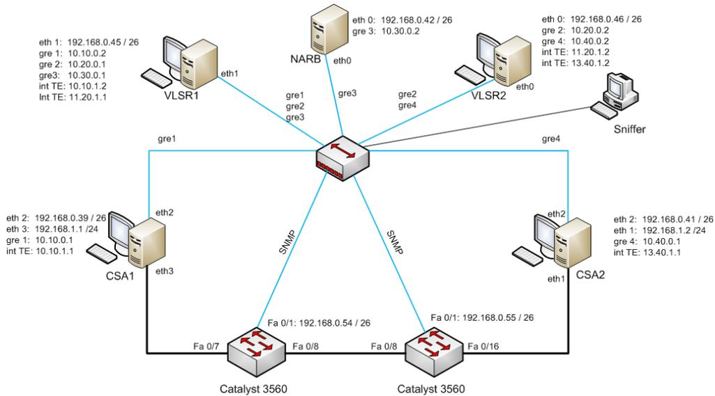
Fig. JA7-2 Second scenario: The extended topology of *KT-GMPLS* network using NARB in intra-domain environment
