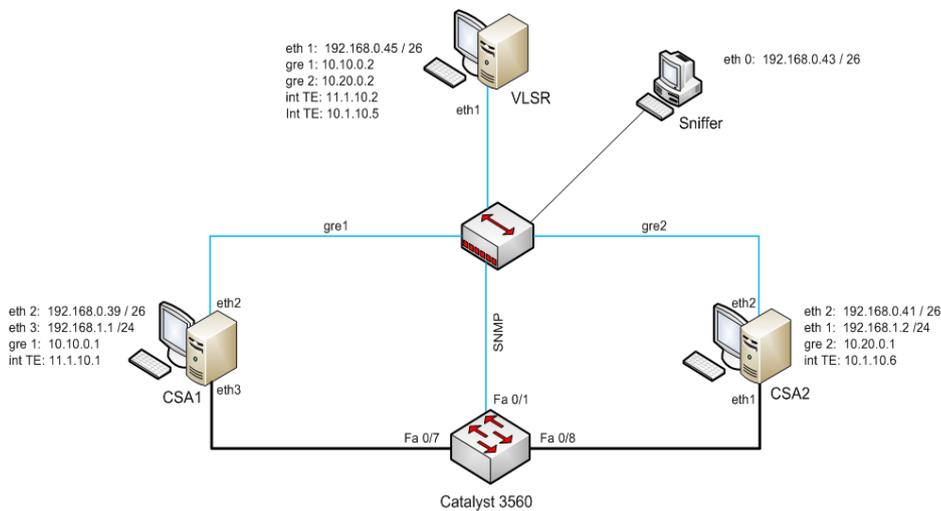
Fig. JA7-1. First scenario: The basic topology of KT-GMPLS
