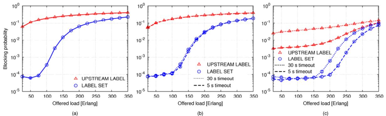
Fig. JA10-3 Blocking probability comparison between the Upstream Label scheme and the Label Set scheme in the (a) NI, (b) AI, and (c) DI scenarios.
