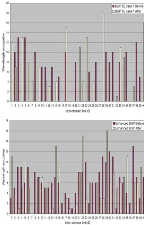
Figure JA2-3 Wavelength occupations before and after re-convergence for BGP TE case 1 and Enhanced BGP schemes
