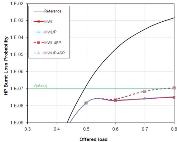
Figure JA9-3 HP burst loss probability as a function of the normalized offered load comparing the reference algorithm with the proposed MWL and MWL/P algorithms.
