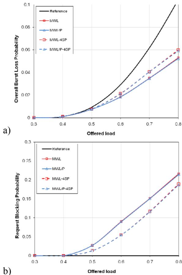
Figure JA9-4 a) overall burst loss probability and b) request blocking probability as a function of the normalised offered load comparing the reference algorithm with the proposed MWL and MWL/P algorithms.
