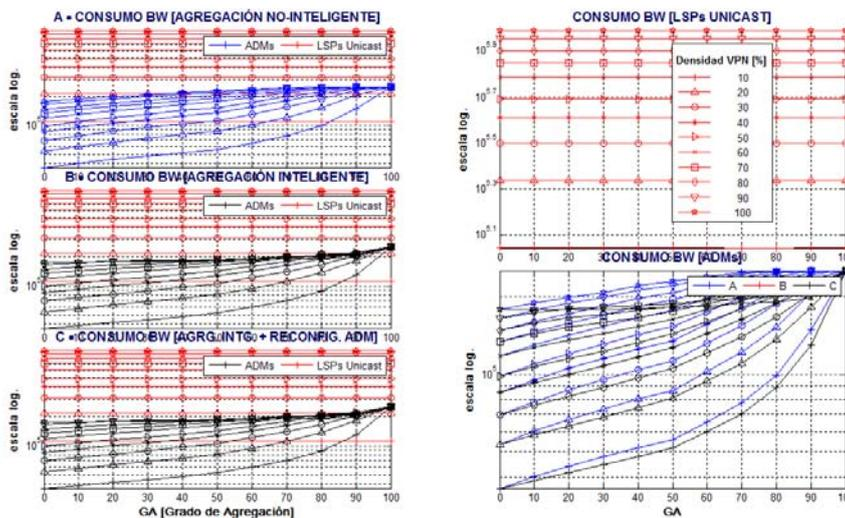
Fig JA5-2 Bandwidth consumption in Tiscali network for 75% of VPLS member density
