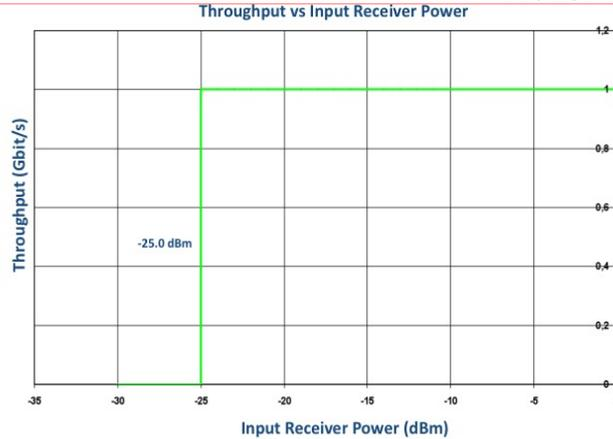
Figure 109: Throughput vs Input Receiver Power in a link 350 km long
