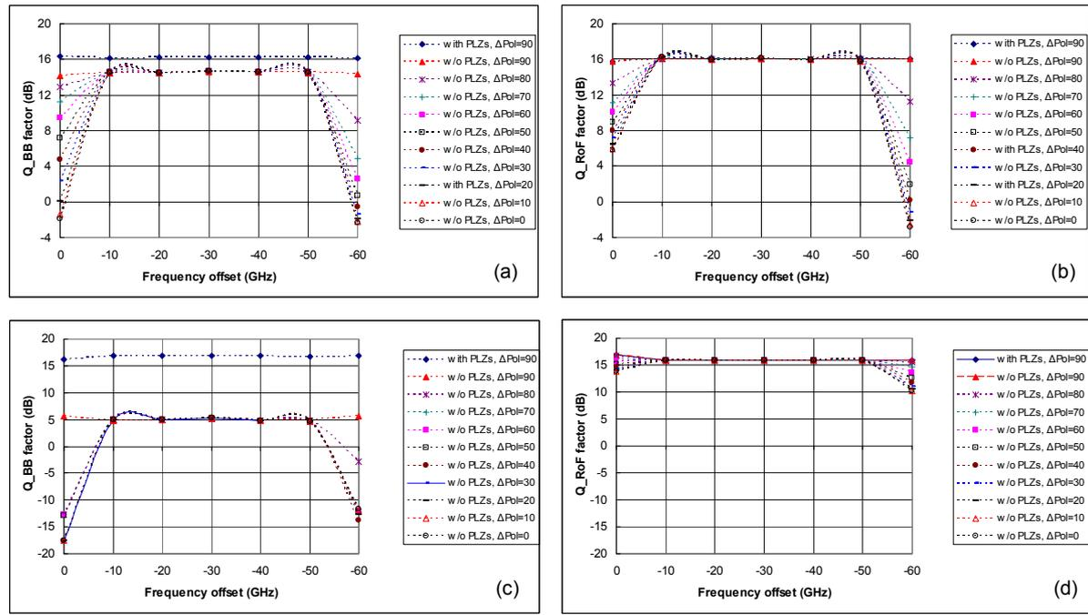
Figure 41:  $Q$ -factor evaluation for different frequency offsets between the carrier of the mm-wave signal and the wavelength-interleaved BB signal and for varying the difference in the SOP ( $\Delta Pol$ ). The BB receiver sensitivity is (a,b) 3-dB (c,d) 15-dB lower than the RoF one
