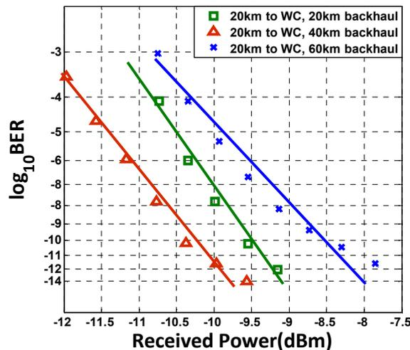
Figure 52. Transmission distance measurements for 20, 40, 60km backhaul
