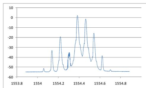
Figure 31. Optical signal after amplification using EDFA, with WiMax modulation signal applied to OSSB generator.
