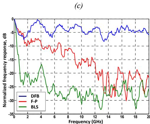
Fig. 46: Measured influence of the optical source linewidth on the frequency response of a (a) 3050 m, (b) 6100 m and (c) 9150 m MMF link.
