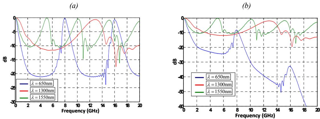
Figure 45: (a) 2km-long MMF frequency response at different DFB ( $W=10$  MHz) source wavelengths. (b) 2km-long MMF frequency response at different FP ( $W=5$  nm) source wavelengths.
