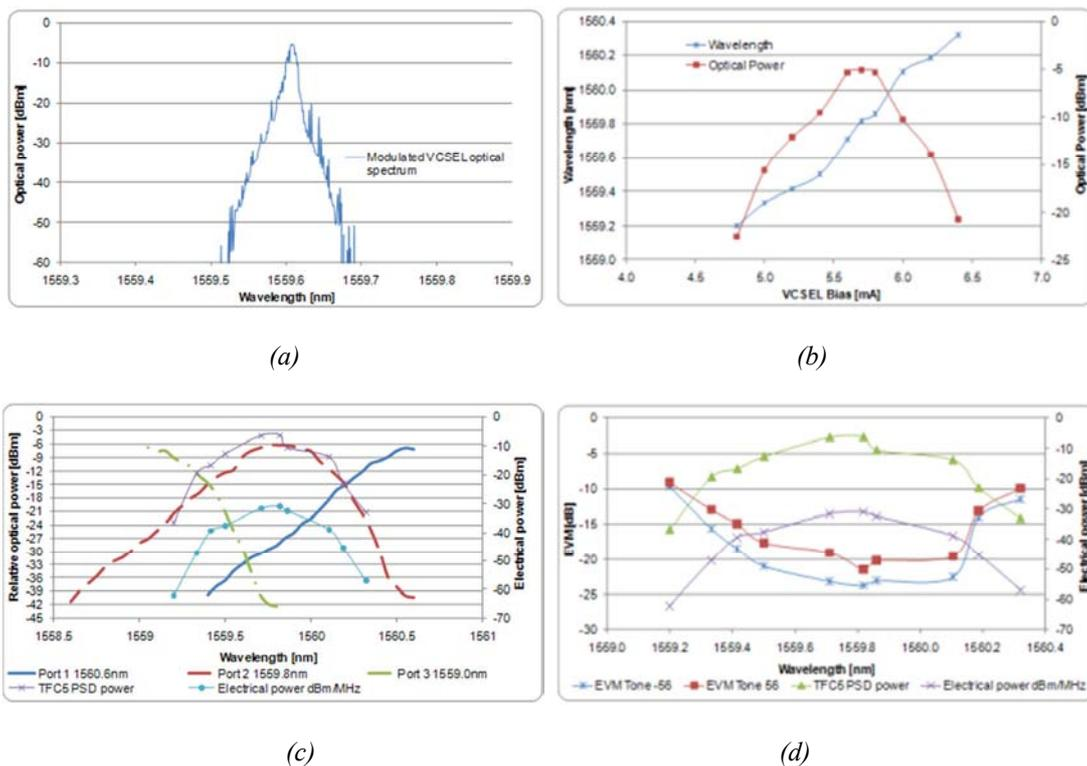
Fig. 7: (a) Directly modulated VCSEL, FM broadening; (b) VCSEL wavelength shift with bias with AWG port 2 optical power; (c) OFDM electrical power detected with changing wavelength after AWG with ports 1, 2 & 3 optical power profiles; (d) EVM of edge tones  $\pm 56$  and their electrical powers variation with wavelength on port 2 of AWG.
