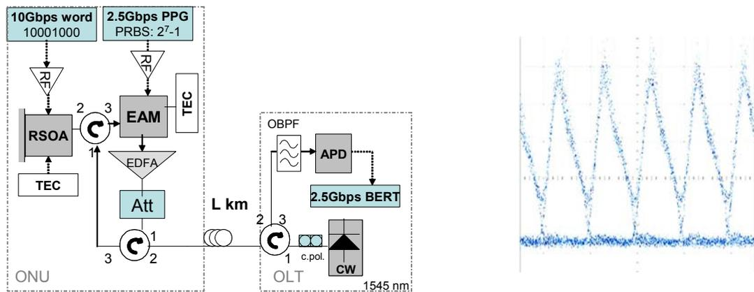
Figure 47. Set up (left) and EAM's output (right) after PRBS of EAM and RSOA synchronization
