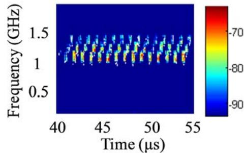
Figure 38: Processed spectrogram of the received UWB signal using TFC1 configuration after photonic-ADC
