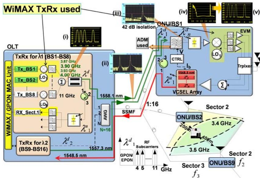
Fig. 9: WiMAX over multi-wavelength, power splitting PONs.
