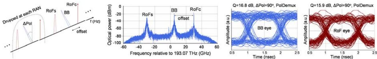
Figure 40: Wavelength division multiplexing and interleaving combined with polarization multiplexing to integrate BB and mm-wave (60 GHz) transmission.
