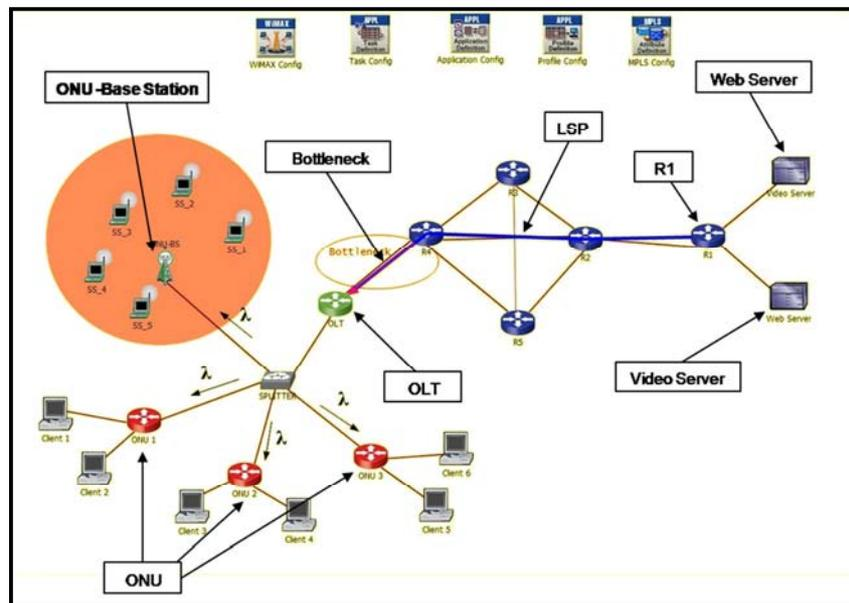
Figure 24 - BS connected to ONU EPON
