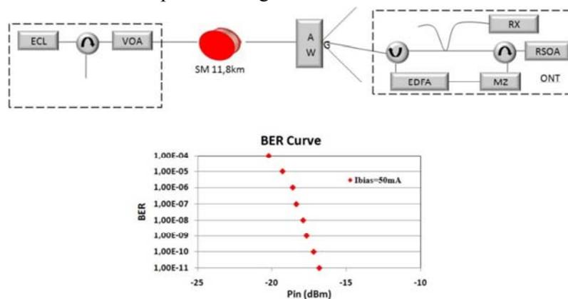
**Figure 2.** WDM PON BER Measurements at ISCOM labs
