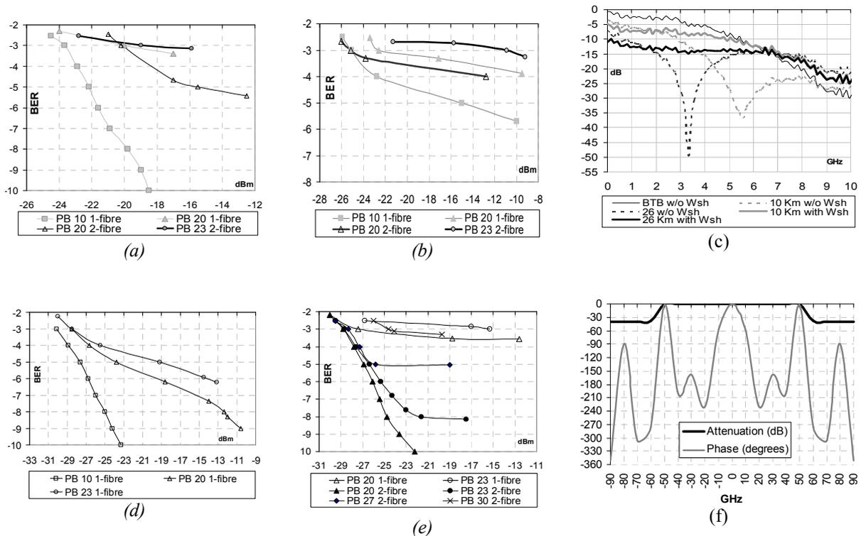
Figure 49. BER with respect optical power for 10.3Gb/s and 10km a) 10.3Gb/s and 26 km b) 5Gb/s and 10km d) 5Gb/s and 26km e). In c) e/o response for BTB, 10km and 26km with and w/o Wsh. In f) attenuation and
