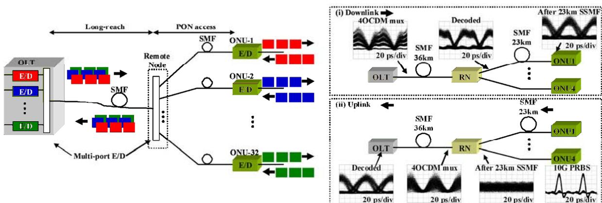
Figure 19. Configuration of the long-reach OCDMA-PON system and experimental setups and results: (i) downlink and (b) uplink.
