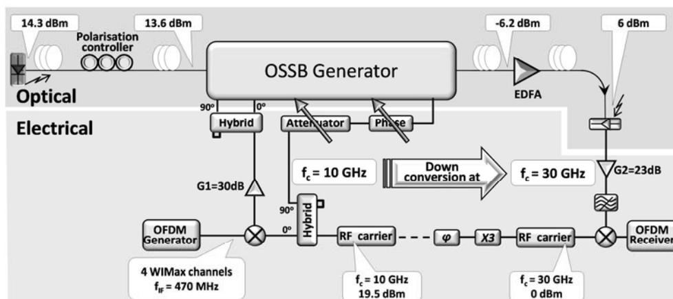
Figure 29. Experimental setup for upconversion
