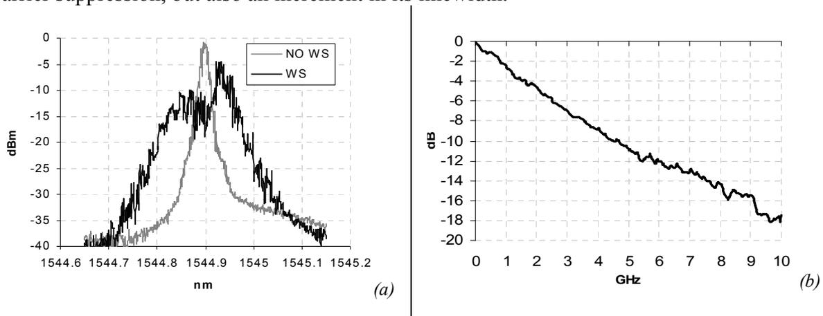
Figure 46. a) Spectrum at the RSOA output with and w/o the electrical modulation b) RSOA e/o BW
