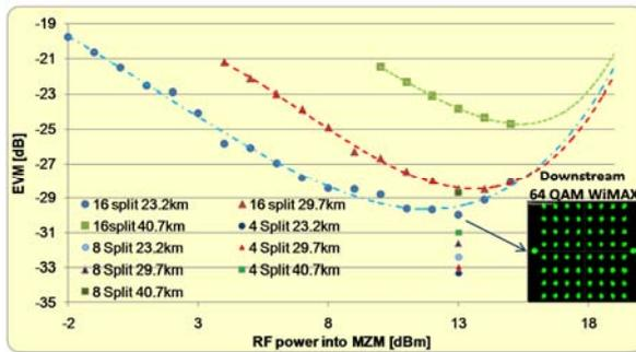
Fig. 10: Obtained EVM for 3.5 GHz WiMAX channel at remote antenna downstream.
