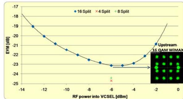
Fig. 11: Obtained EVM at the WiMAX OLT receiver for 3.5 GHz channel upstream.
