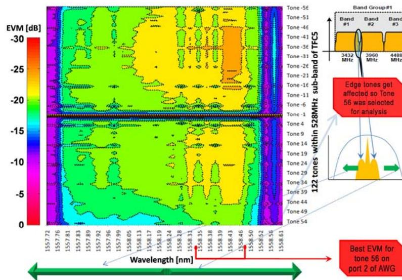
Fig. 8: EVM fluctuations for all OFDM tones with variation in wavelength.
