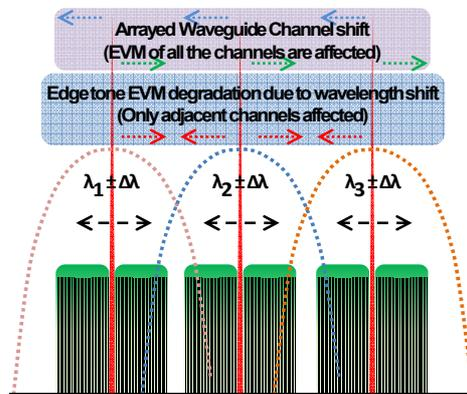
Fig. 6: EVM of affected edge tones due to wavelength shift
