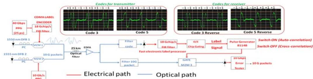
Fig. 20 (a) Experimental setup for the 18 Gchip/s ECDMA label recognition system and optical label forwarding. The codes used are shown (time axis 200 ps/div).
