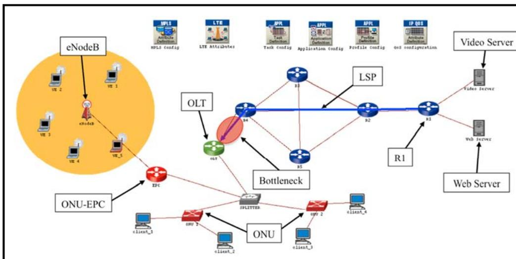
Figure 26. EPC connected to ONU EPON
