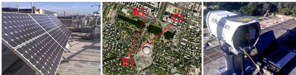
**Figure 1.** Wireless Set Up: Photovoltaic Station to supply the FSO Heads [Left], Test Bed Area [Center] (A and C are ISCOM premises while B is a Tower 60m tall also called “the mushroom”, The FSONA FSO system [Right])
