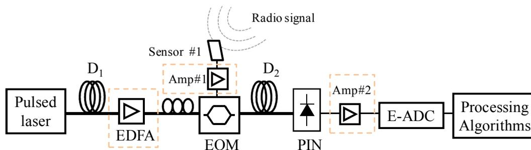
*Figure 37: Proposed single-channel Ph-ADC architecture with engineered optical and electrical amplification*
