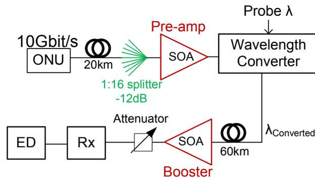
Figure 51. Schematic of a wavelength converted PON with 60km backhaul section, with an amplifier before the receiver to boost the signal power level
