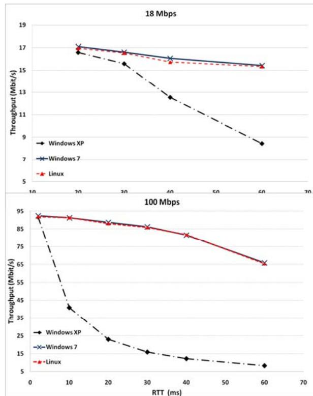
Figure 23 TCP connection Throughput evaluation.
