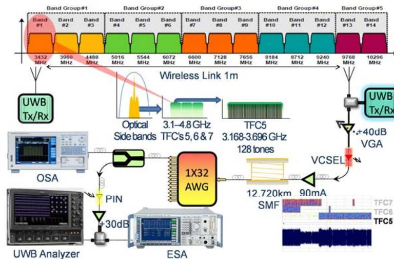
Fig. 5: Performance monitoring system setup in laboratory
