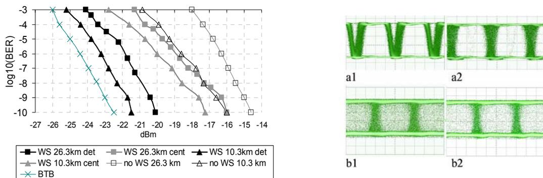
**Figure 48.** BER results (left) and Eye diagrams for 26.3km after APD with a) and without b) WS, with the filter detuned (1) and centered (2) for the same optical power (-20dBm) (right).
