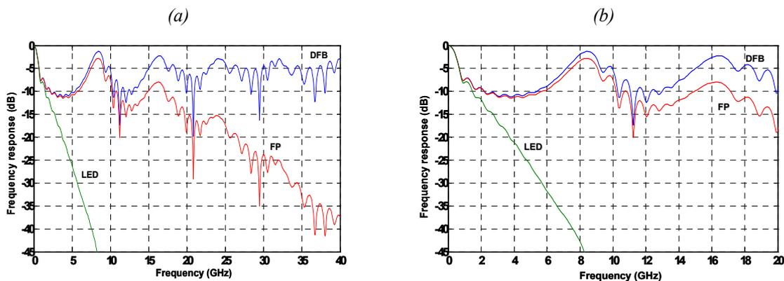
Figure 43: (a) Influence of the temporal coherence of the source on frequency response for a fibre link of  $L=3\text{Km}$ . (b) Influence of the temporal coherence of the source on frequency response for a fibre link of  $L=6\text{Km}$ .
