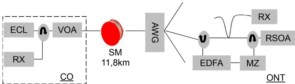
Figure 28: scheme of the WDM PON
