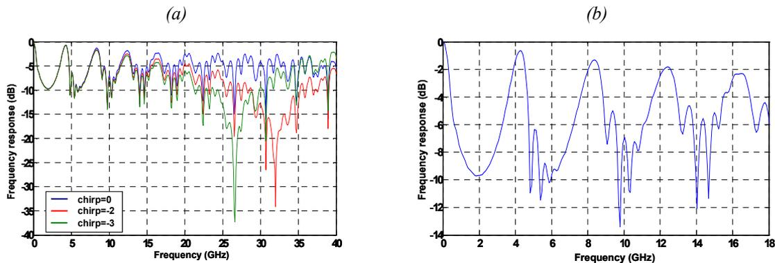
Figure 44:- (a) Frequency responses and Carrier Suppression Effect for different values of the source chirp for a fibre link of  $L=6\text{Km}$ . (b) Zoom of the frequency response considering the condition  $\text{chirp}=0$ .
