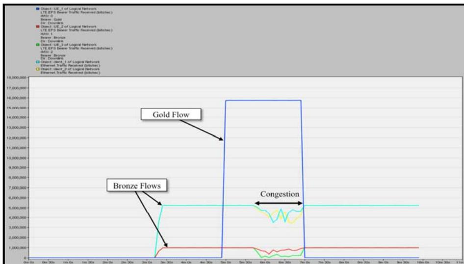
Figure 27. Traffic received with congestion on the link before OLT
