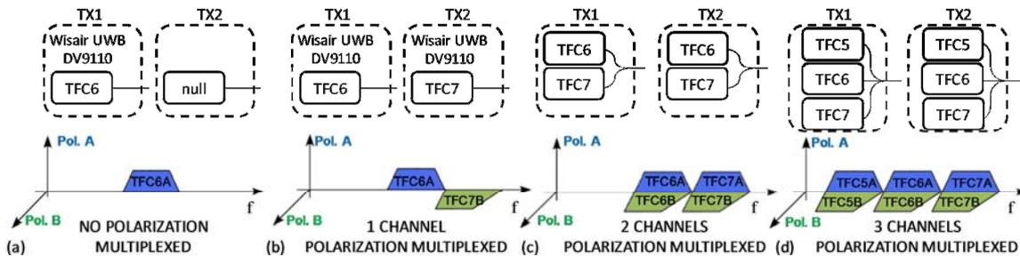
Figure 35: Transmitter configurations and spectrum schemes: (a) without PM, (b) 1 channel PM, (c) 2 channels PM and (d) 3 channels PM
