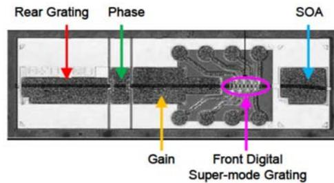
Fig. 53 Top view of a DS-DBR laser chip
