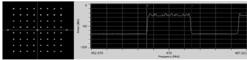
Fig. 32. Measured frequency spectrum and constellation in back-back WiMax Tx-Rx configuration for establishing baseline RCE (-36.726 dB).
