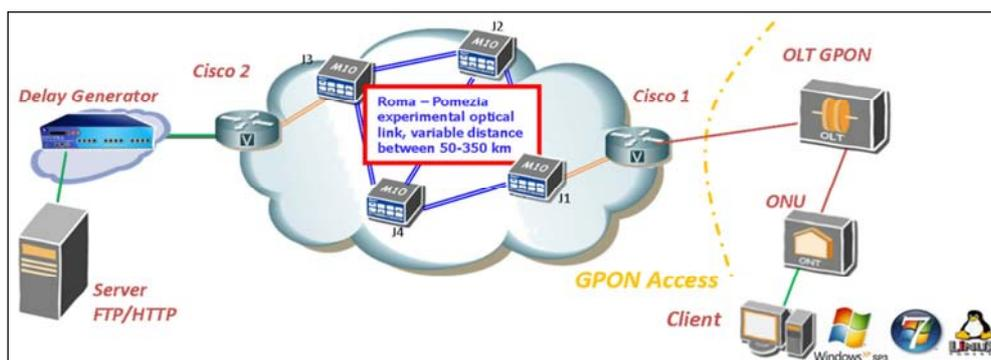
Figure 22 Test Bed Design
