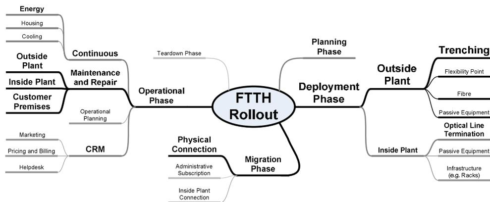
Figure 13: Capital and operational costs for the rollout cycle of an FTTH network [2]
