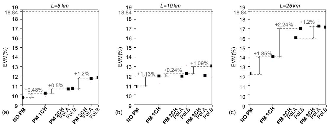
Figure 36: Experimental EVM results in TFC6 for different PM configurations and different FTTH paths: (a)  $L=5$  km, (b)  $L=10$  km and (c)  $L=25$  km
