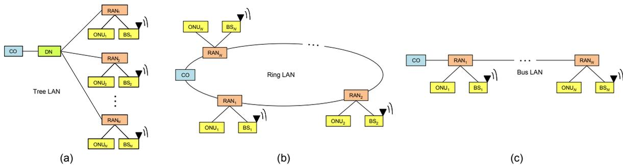
Figure 39: Integrated access network architectures. (a) Tree (b) ring and (c) bus topologies. CO: central office, DN: distribution node, RAN: remote access node, ONU: optical network unit, BS: base station.
