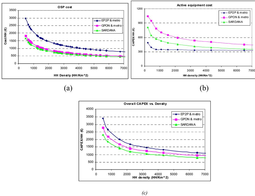
Fig. 17: a) OSP equipment CAPEX/user vs. HH density, b) Active equipment CAPEX/user vs. HH density c) Overall CAPEX/user vs. HH density
