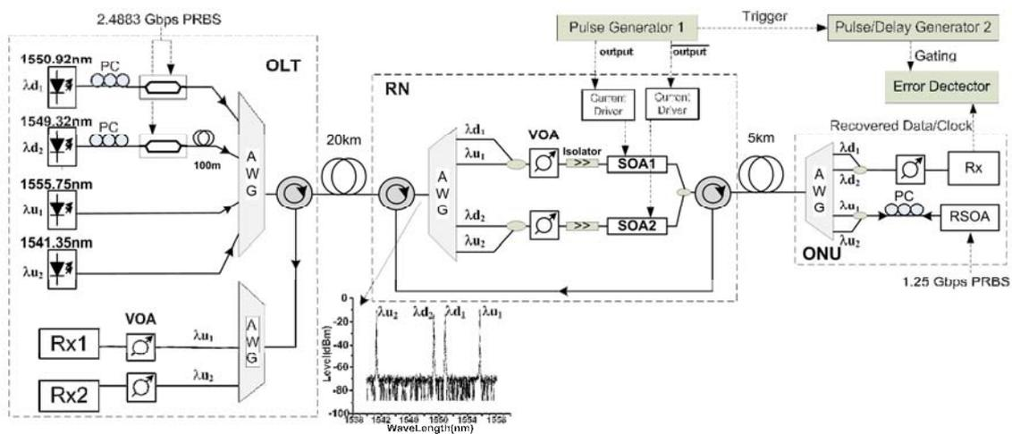
Figure 56. Experiment Setup
