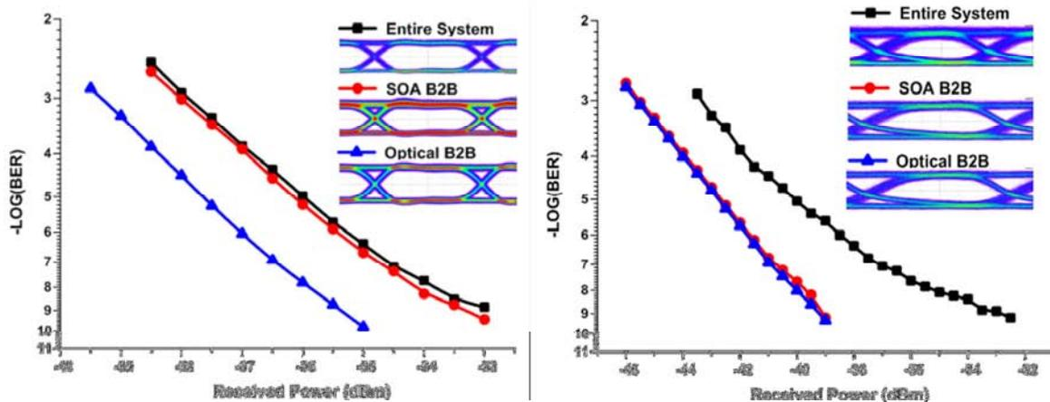
Figure 58. 2.5 Gbps downstream BER tests (left), 1.25 Gbps upstream BER tests (right)
