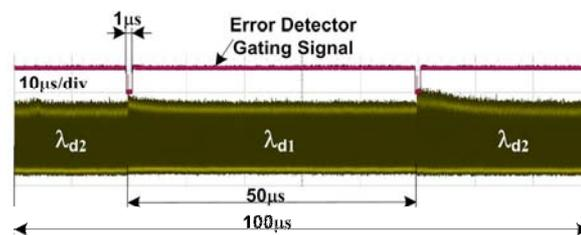
Figure 57. Time traces of optical power at ONU Rx and error detector gating signal.
