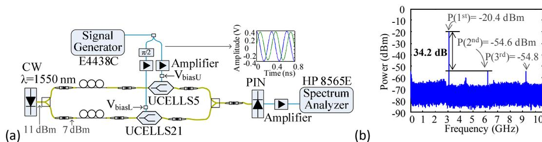
Figure 34: (a) Experimental setup for dual parallel Y coupled linearized characterization, and (b) Measured electrical spectrum for dual parallel Y coupled linearized proposed architecture.
