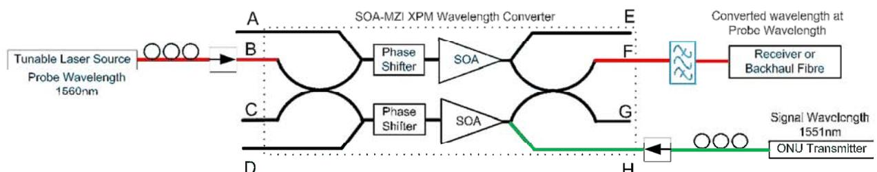
Figure 50 SOA-MZI wavelength converter utilising cross phase modulation, the dash line section contains the integrated SOA-MZI XPM Wavelength converter
