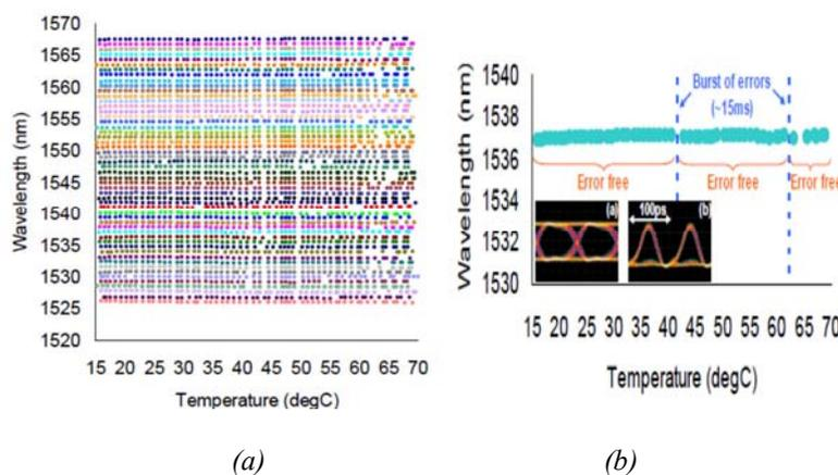
Fig 54. (a) Coverage of C-band uncooled WDM channels (53 channels with 100GHz spacing). (b) Wavelength stability and transmission performance of a representative channel over a temperature range from 15 to 70°C. Including signal eye diagram in NRZ operation, and RZ eye diagram for BER measurements (insets).
