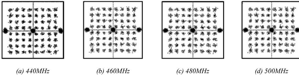
Fig. 33. Measured constellation for the  $4 \times$  WiMax channels at 440 MHz, 460 MHz, 480 MHz and 500 MHz (RCE measured: -19.438 dB, -20.22 dB, -20.033 dB and -20.459 dB, respectively).
