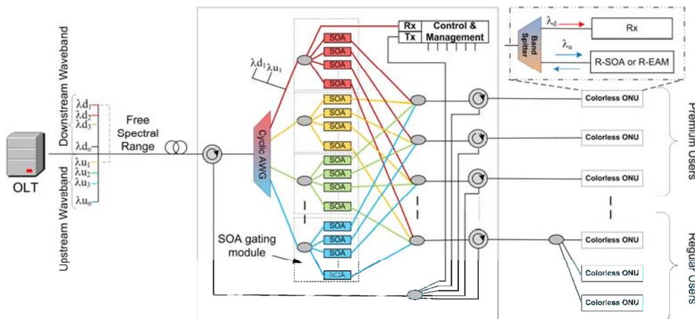
Figure 55. Active routing optical access network architecture
