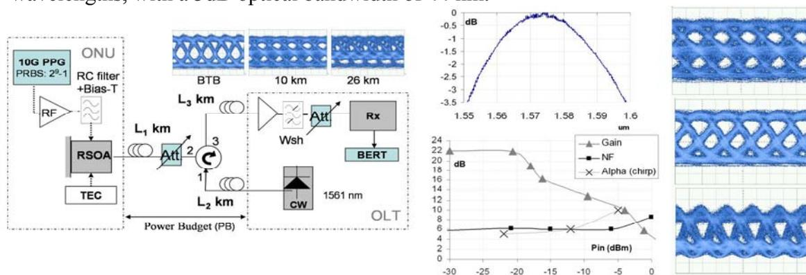
Figure 48. **Left:** Set up and eye diagrams in BTB, and after 10km and 26 km. **Middle up:** RSOA ASE curve. **Middle bottom:** RSOA's gain, noise factor and chirp respect optical power. **Right:** eye diagram comparative after 10km with a simple flat filter centred (top), a filter detuned (middle), the flat filter centred with a specific phase (bottom)
