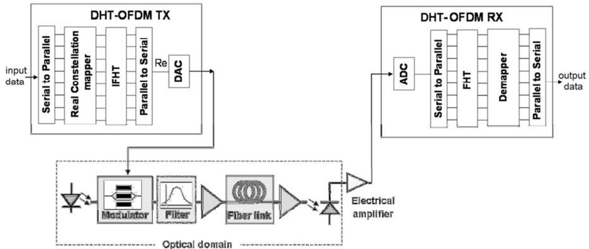
Figure 18. Optical DHT-based OFDM system. The OFDM-modulation and demodulation are performed in the electrical domain by using an  $N$ -order inverse FHT and forward FHT, respectively. The optical detection is direct. The components in grey are in the optical domain.
