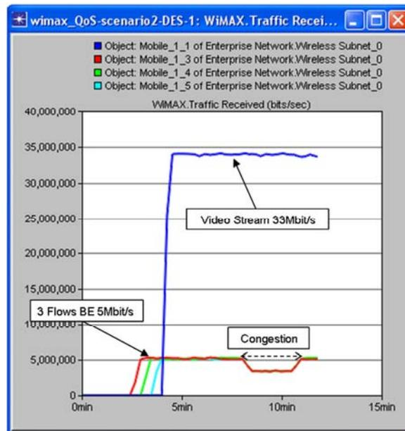
Figure 25 - Traffic received with congestion on the link before WiMAX cell
